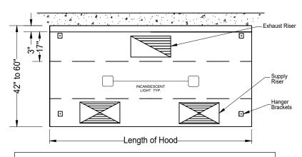
It is the responsibility of the architect/owner to ensure that the hood clearance from limited-combustible and combustible materials is in compliance with local code requirements
