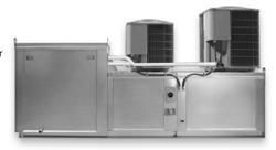
One benefit of this unit is the multiple cooling stages. Multiple cooling stages increase the efficiency by not using 100% of the cooling capacity when this is not needed, thus allowing lower energy usage. An internal make-up air cooling thermostat automatically energizes the first stage when cooling of the make-up air is required. The same thermostat has a built in adjustable differential to energize the second stage of cooling when required.
