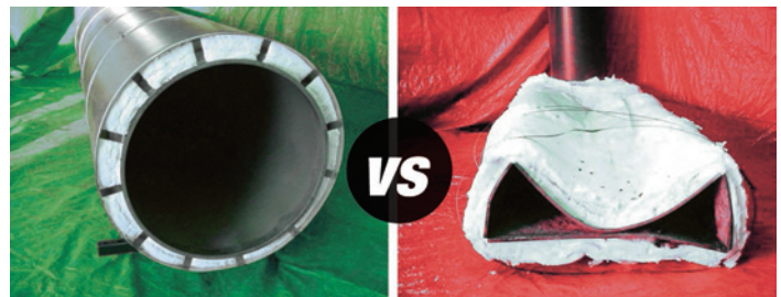
ZVS after 2000°F (simulated grease fire) for 30 minutes.
